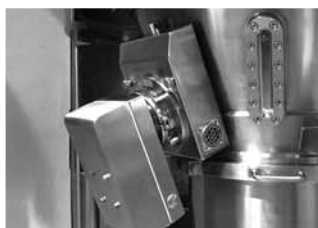
NIR sensor on fluid bed
