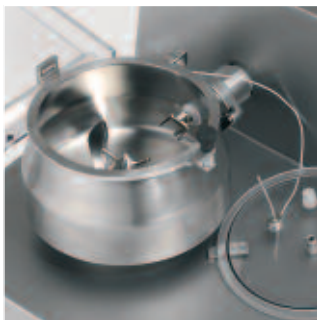
Mixing bowl with temperature probe in the lid.
