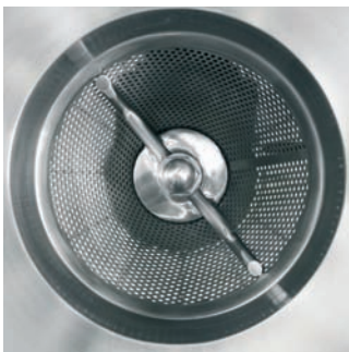
The material can be calibrated during discharge by using a sieving mill below the outlet.
