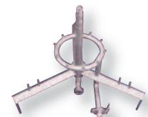
Washing stand for drums. Note dual channel spray systems, one for washing and one for USP/DI rinse water
