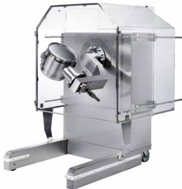
Multi-Purpose, Pilot size unit for Drums, V-shells & Bins
