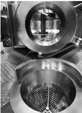
Opened discharge valve and Tool-lift of the mixer-granulator.
