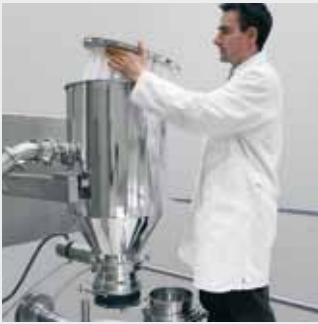
Excellent access to all plant components is shown here for the vacuum conveyor to discharge the dryer.
