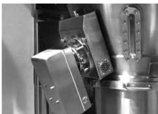
NIR sensor on fluid bed
