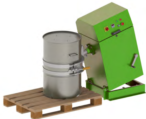
CM type MIXOMAT, position "down"
