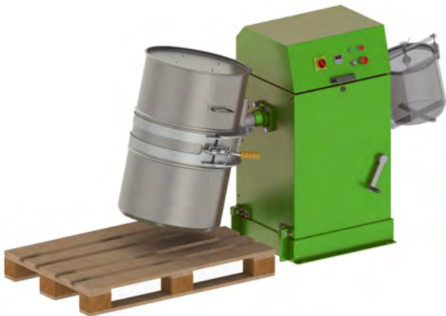
CM type MIXOMAT with second holder, position "up"
