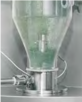
Wurster-Bottom-Spray: Coating in the MINILAB.
